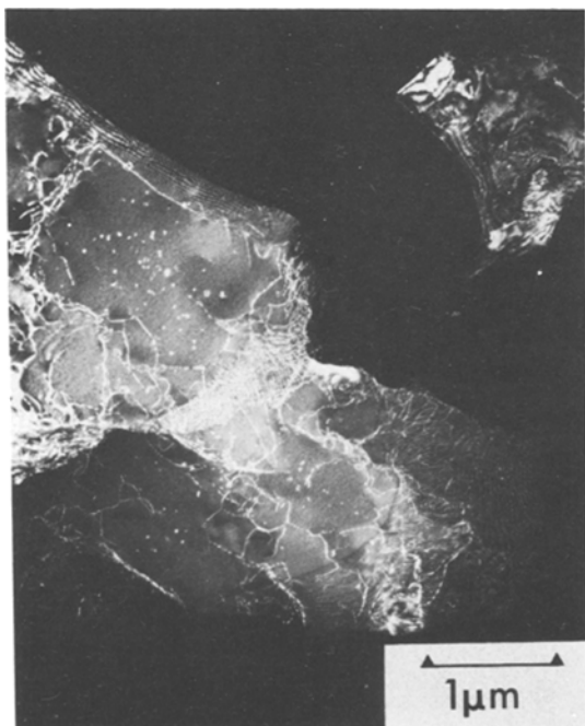
Figure 2 The microstructure of the cold-rolled material. Dark-field electron micrograph taken under weak beam diffraction conditions.
