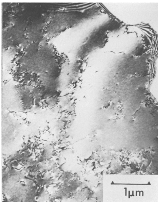
Figure 6 The microstructure after 100% tensile deformation at 400° C. Note the increased grain size and higher dislocation density within the grains compared to Fig. 3.
